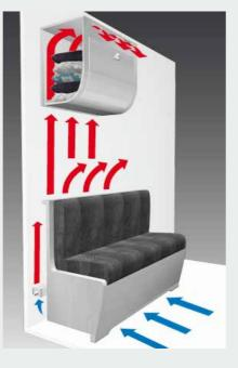
This is how it should be when the hot air from the convectors flows up behind the sofa and upper cabinets.
